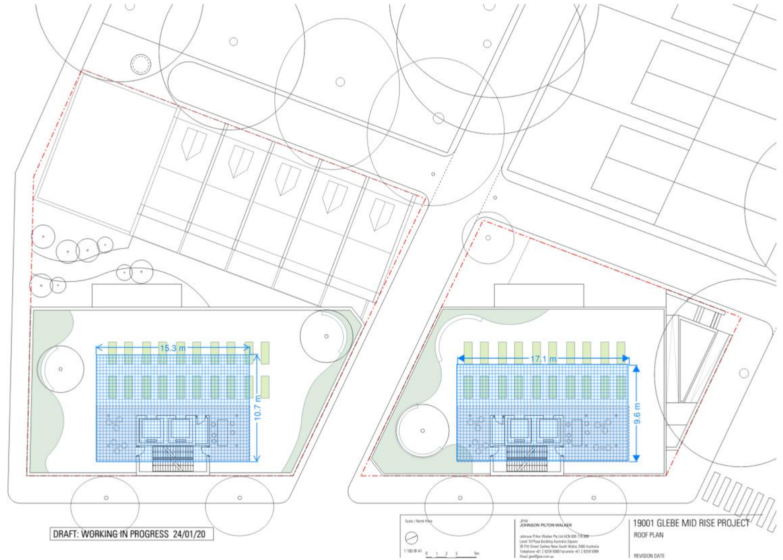
Figure 13 – Rooftop Solar PV assessment
